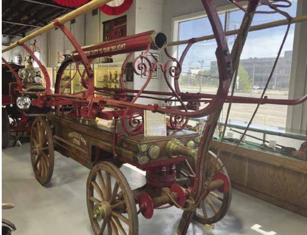
Button 1855 hand engine. Note the motto on the tube holder of “squirrel tail,” “piano-box” style wood tub, “hayrack” pump brakes folded-up in the stored position, and rope reels at front for hauling engine. Photo courtesy Curt Peters, Vintage Fire Museum, Jeffersonville, IN.
