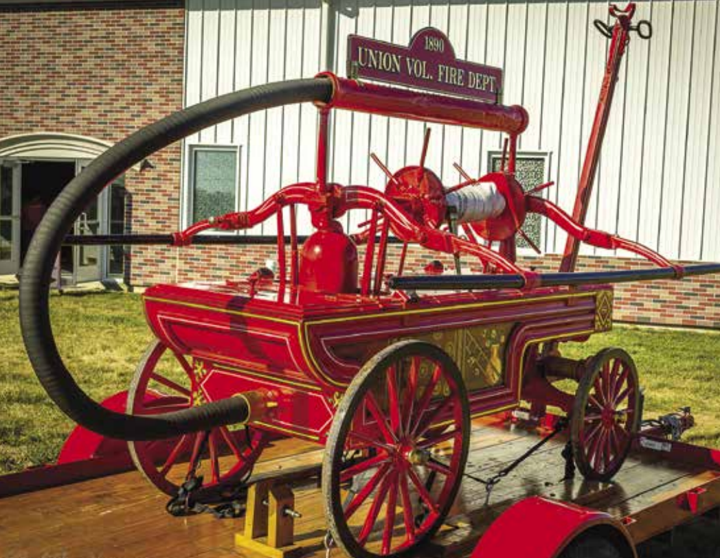
Restored L.M. Rumsey Mfg. Co. 1890 hand engine. Note: “piano-box” style tub, “squirrel-tail” draft hose, and center mount hose-reel. Courtesy Don Wilmesher and Union Fire Protection District, MO. Photo by Gail Hagans.
