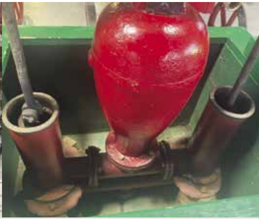
Close-up of handtub pump engine box, twin cylinders, and air chamber on discharge in the middle. Photo courtesy Curt Peters, Vintage Fire Museum, Jeffersonville, IN.
