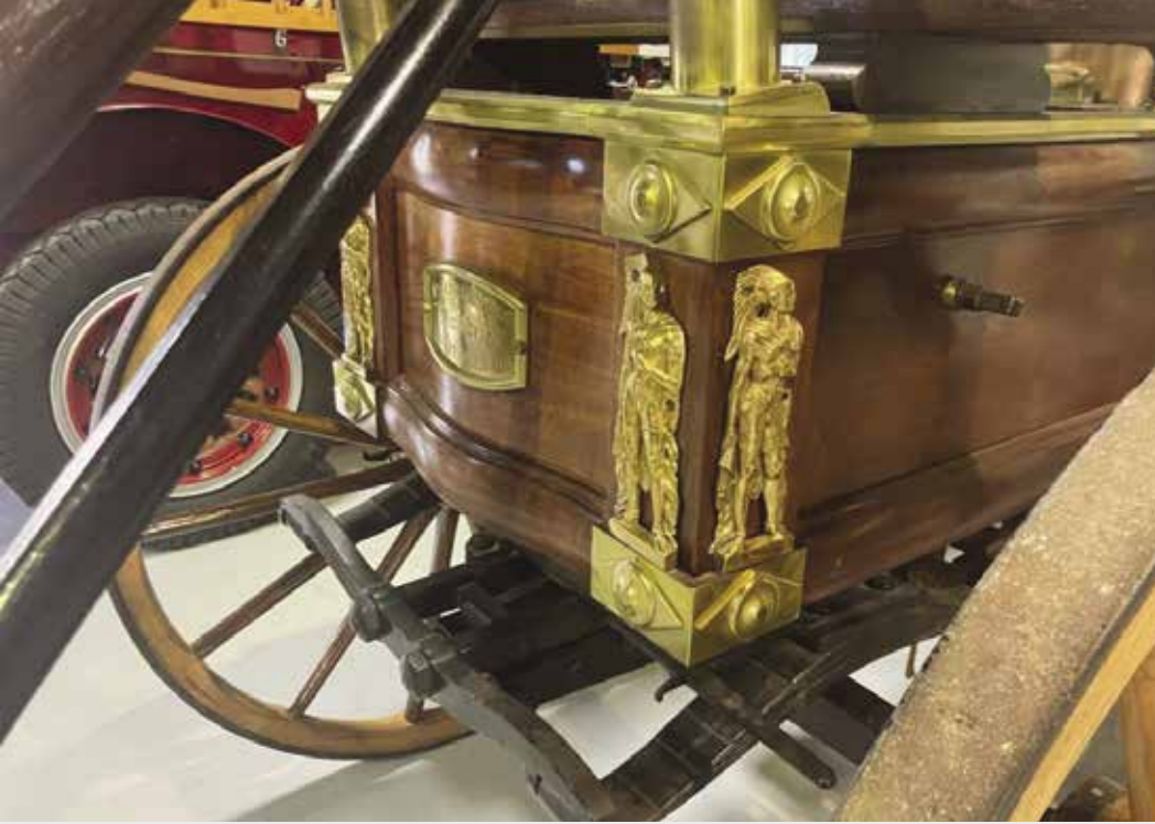
Close-up of polished wood "tub" and intricately detailed brass work of Jeffers Co. "Mohawk" hand engine. Photo courtesy Curt Peters, Vintage Fire Museum, Jeffersonville, IN.
