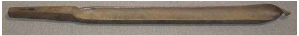
Water Pod Auger 1750, used for drilling waterways in logs. Photo from the Davistown Museum/Maine Memory Network,
