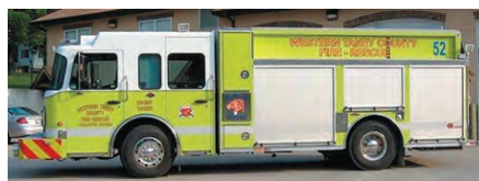
Engine 52 of WTCFPD was designed by the fire district staff to function as a tanker or engine and carries basic wildland tools and minimal rescue equipment.
