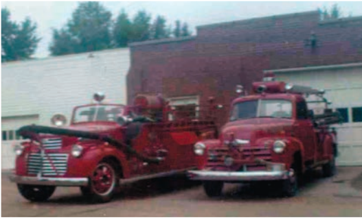
1942 GMC/CENTRAL 500 GPM PUMPER AND 1948 CHEVY HOME BUILT WITH THE BED FROM THE ORIGINAL 1927 CHEVY FRONT MOUNT
